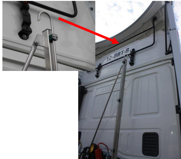
Truck blow-off pipe
